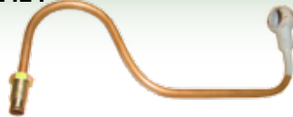
Pipe 35 4 Cylinder Filter to Injector Pump
